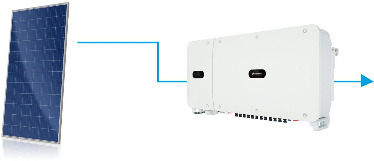
Where three or more strings are wired in parallel, either in a DC junction box or internal to the inverter it is essential that each string has its own string fuses, on both polarities. This will avoid reverse currents destroying modules in the event of a short circuit. These string fuses would typically be inside the inverter or in the DC junction box, depending on the manufacturer and inverter model chosen.
